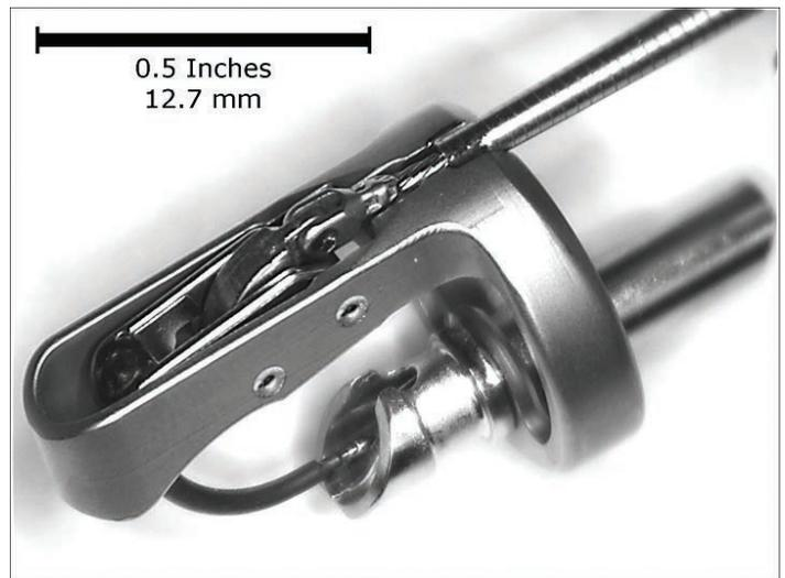
Apollo Endosurgery Overstitch System, with 12 laser welded joints, seven of which are visible in this photo.
